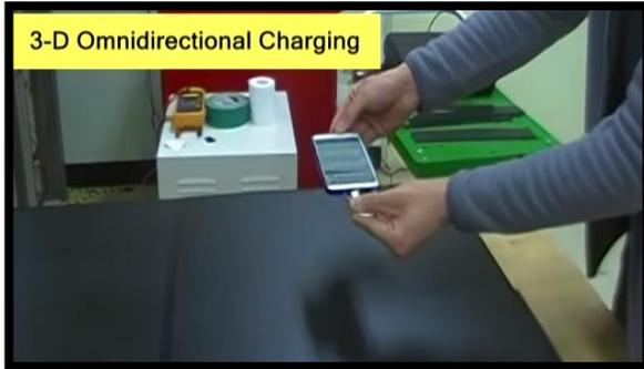
Wireless charging is becoming commonplace with many smartphones coming with the technology built-in and some businesses offering compatible charging pads. However, all existing systems still require you to place the phone on the pad in a certain way so the coils can line up. A team of researchers at Korea Advanced Institute of Science and Technology (KAIST) have developed a prototype for a wireless charging system that works at distances up to half a meter and in any orientation.
